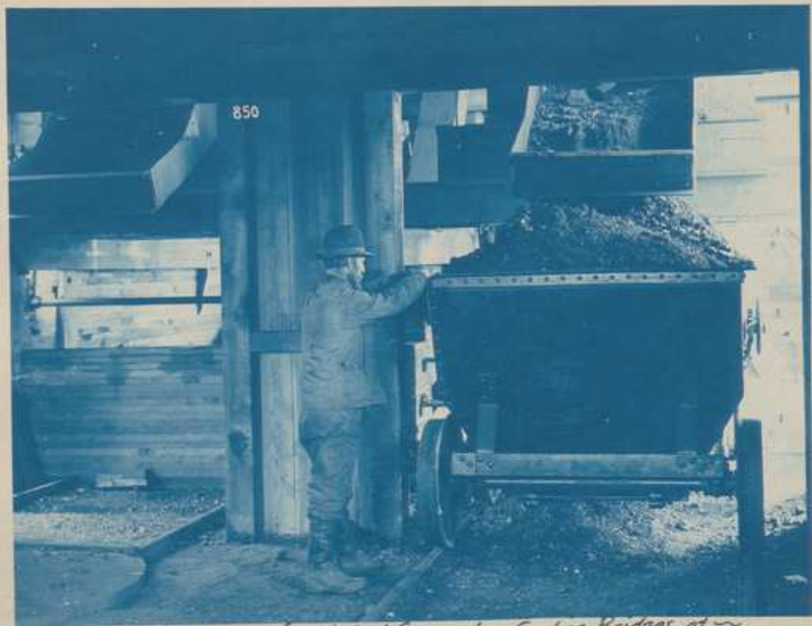
~Bottom Dumping (2Ton) Coal Car used on Cooling Bridges at ~ Croton & Lyons Stations - N.Y.C. & H.R.R.R.~
