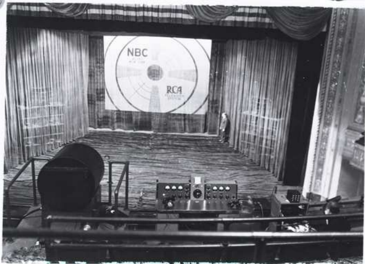
Fig. 4 Projector and Control Equipment as Viewed from Stage.
