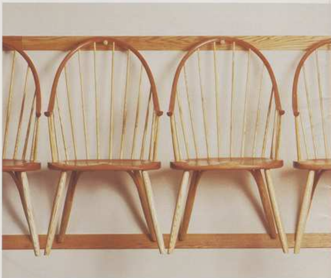
Continuous Arm Chairs drying between coats of oil. Rubbed finish takes 7 to 10 days.
